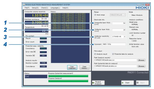
1 Enter the composite layer thickness in the [Composite layer thick. [µm]] field.
