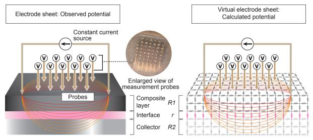
(It doesn't matter whether the electrode sheet that is measured is coated on one side or both sides. The composite layer resistivity and interface resistance on the probed surface are output.)
