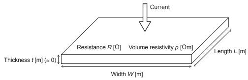
Figure: Definition of surface resistivity
