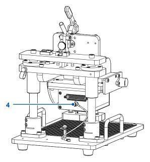
4 Connect the grounding cable on the rear of the RM9003 Press Unit to the ground terminal on the RM9004 Test Fixture.
