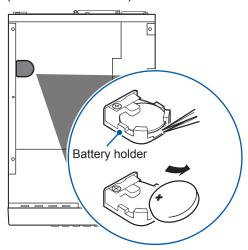
Insert the tweezers into the space between the battery and the battery holder and remove the battery while lifting up on it, as shown in the figure.
