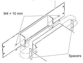
2 Insert spacers on both sides of the RM2611 Electrode Resistance Meter and then install the rack-mounting hardware with M4 × 10 mm screws.
