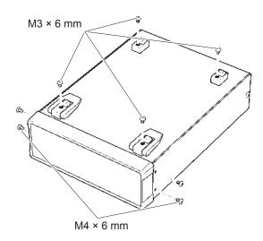
1 Remove the screws from the RM2611 Electrode Resistance Meter's support feet (on the bottom) and side cover (total of 4 on the sides at the front).
