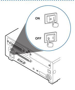
Place the RM2611 Electrode Resistance Meter's main power switch (on the rear of the instrument) in the ON (|) or OFF  $(\circ)$  position.
